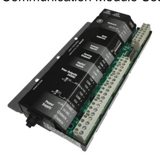
**EVCB14NIT4X** (4 TRIACS / pressure independent / external motor) **EVCB14NDT4X** (4 TRIACS / pressure dependent / external motor)
